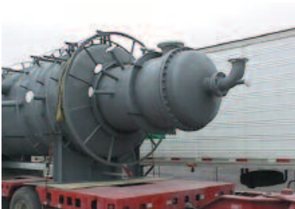
Reaction furnace with acid gas burner ready for shipment
